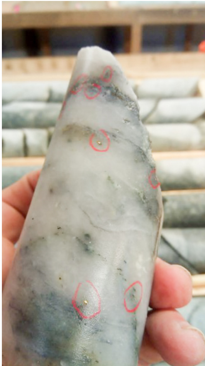
Figure 3: AUDD0078: Multiple 1-2mm flecks of visible gold in laminated quartz-tourmaline-gold vein within strongly sericite-altered Quartz Feldspar Porphyry. Sample 40cm at 117 g/t gold from 21.3m. Diamond core NQ diameter (image 47.6mm width).
