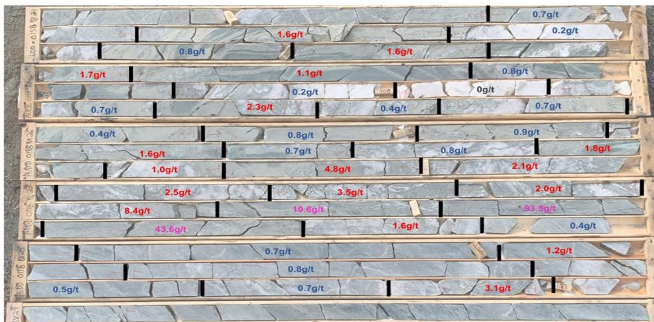
Figure 9: AUDD0158: New Discovery. 102.65m to 123m. Sericite-ankerite-pyrite altered intermediate dyke within sericite-ankeritepyrite altered Quartz-Feldspar-Porphyry. Alteration to the selvage of and is related to multiple sheared Quartz-Ankerite-Pyrite veins. Interval is 20.4m @ 5.3g/t Gold including 2.2m @ 39.3g/t Gold from 116m.
