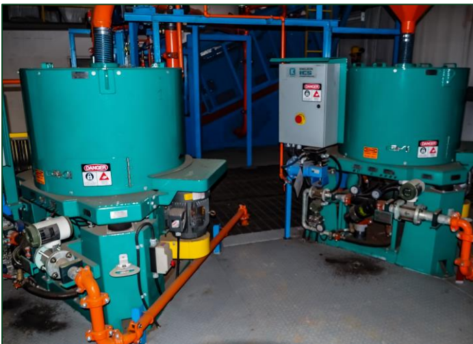
Image 3: Knelson concentrators at the Pickle Crow plant
