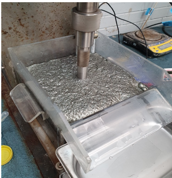
Plate 1: Nickel Cleaner Flotation Test
