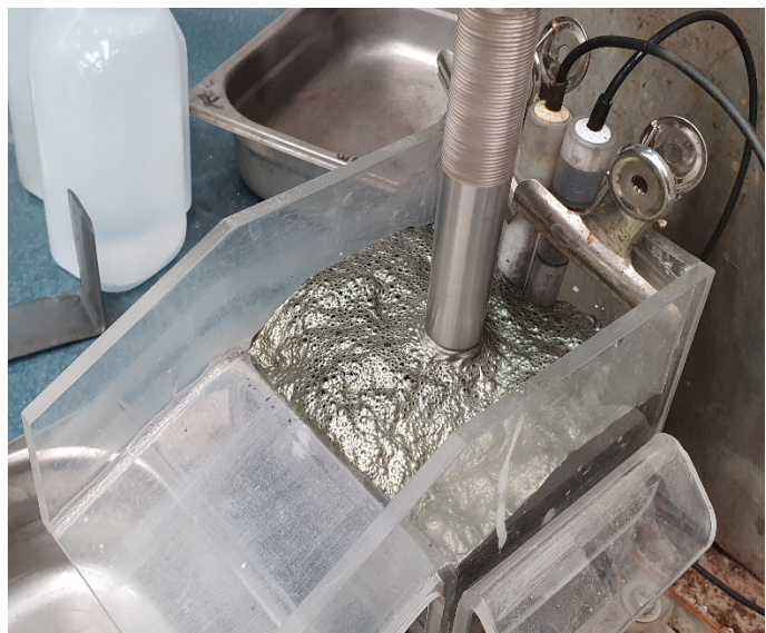
Plate 2: Copper Cleaner Flotation Test
