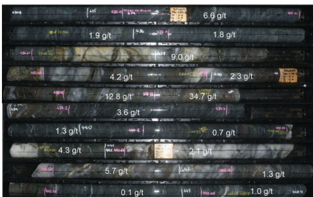
Figure 19: Bellevue South Lode diamond core hole DRDD191 situated above the Viago Lode high-grade mineralization associated with ~5% semi-massive pyrrhotite, trace disseminated chalcopyrite and fine-grained visible gold.
