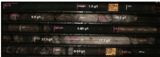
Figure 15: SOUTHERN STEP OUT diamond drill core from DRDD273, high-grade lode mineralization confirmed at the new DHEM plate at the southern extent of the currently tested strike of Deacon; 10% pyrrhotite, trace chalcopyrite and trace visible gold mineralization.
