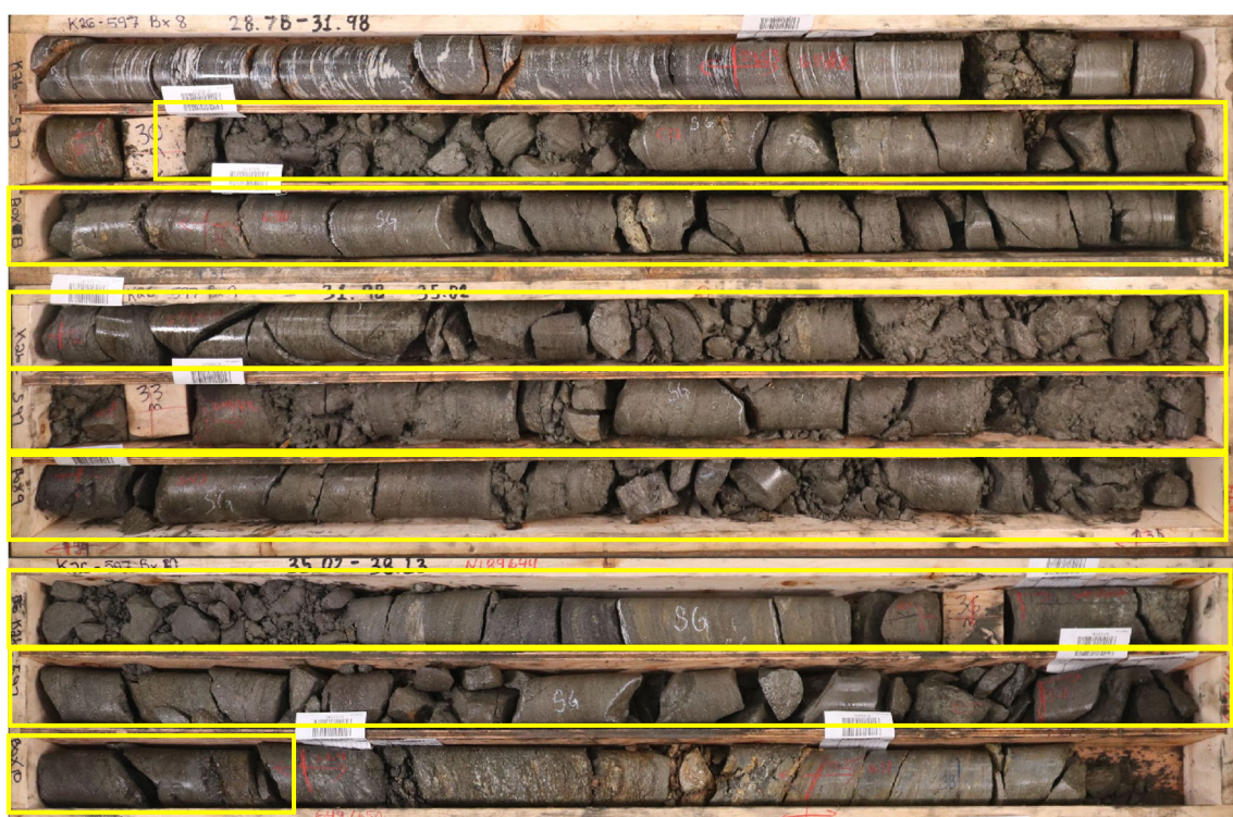
Photo 4: Hole K26-597 (Rhyolite Peak) highlighted interval of 7.4m (7.2m true width) @ 179g/t Ag, 6.9% Zn, 1.1g/t Au, 0.6% Cu, 1.2% Pb from 30.0m, including: 3.0m (2.9 true width) @ 347g/t Ag, 6.2% Zn, 1.7g/t Au, 0.6% Cu, 1.7% Pb from 33.0m
