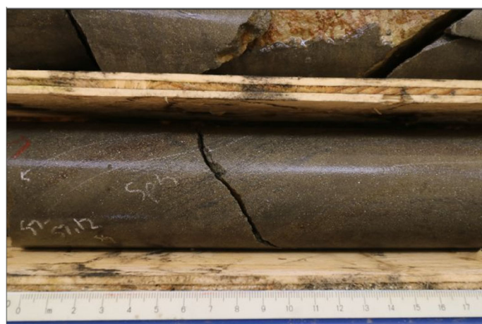
Photo 2: Hole K26-601 (Rhyolite Peak) from 57.0-57.2m. Massive pyrite with a weak foliation, bands of red brown sphalerite parallel to foliation planes. Assay results returned from this sub-interval (57.0m – 57.55m) returned 461 g/t Ag, 9.2% Zn, 1.5g/t Au, 0.2% Cu and 4.8% Pb
