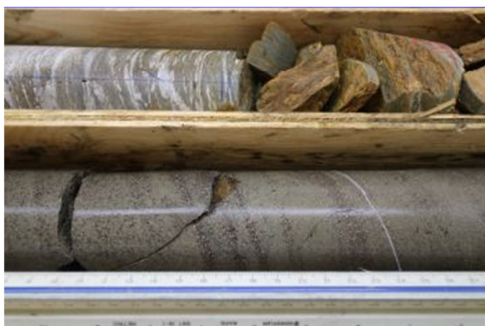
Photo 1: Hole K26-601 (Rhyolite Peak) from 55.1-55.3m. Massive pyrite with a weak foliation, bands of red brown sphalerite parallel to foliation planes. Trace amounts galena, locally seen intergrown with/at margins of sphalerite stringers. Assay results returned from this sub-interval (55.1m – 56.0m) returned 284 g/t Ag, 10.0% Zn, 2.4g/t Au, 0.2% Cu and 2.3% Pb
