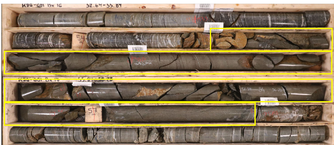
Photo 7: Hole K26-601 (Rhyolite Peak) highlighted interval of 3.1m (3.0m true width) @ 306g/t Ag, 8.1% Zn, 1.7g/t Au, 0.1% Cu, 3.0% Pb
