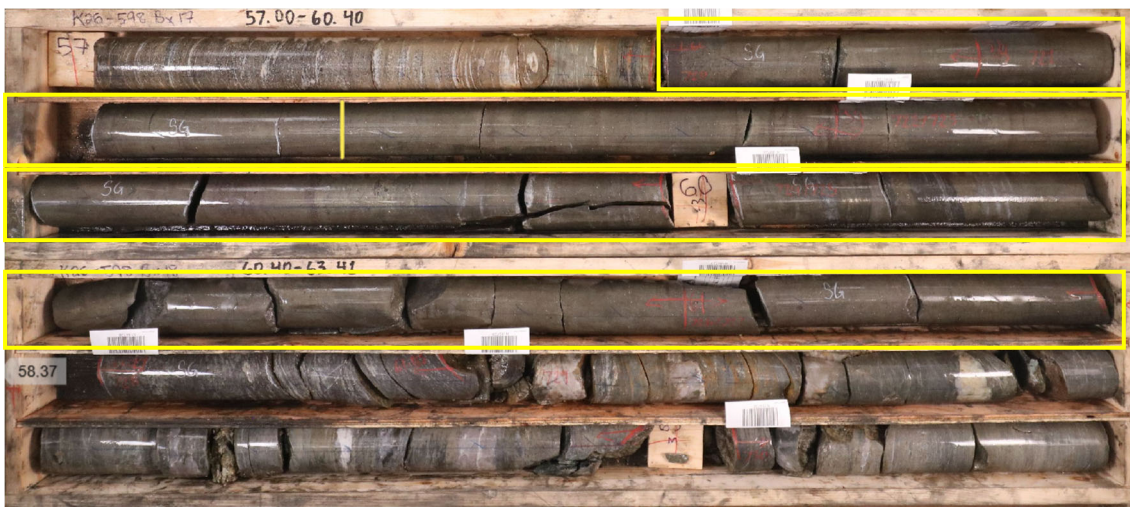
Photo 5: Hole K26-598 (Rhyolite Peak) highlighted interval of 5.2m (5.1m true width) @ 233g/t Ag, 9.0% Zn, 1.7g/t Au, 0.4% Cu, 2.6% Pb from 56.7m including: 3.4m (true width) @ 331 Ag, 12.5% Zn, 2.5g/t Au, 0.5% Cu, 3.7% Pb from 58.0m
