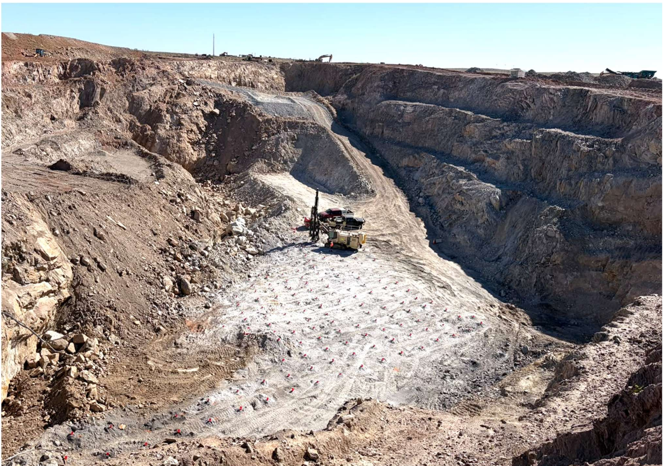
Figure 2. Pinnacles open pit with blast pattern for mining of the now exposed high grade ore within pit floor
