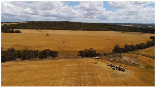
Figure 1. Drilling at Yarabrook Hill. Diamond rig in the foreground, RC rig in the background with Yarabrook Hill forming the skyline.
