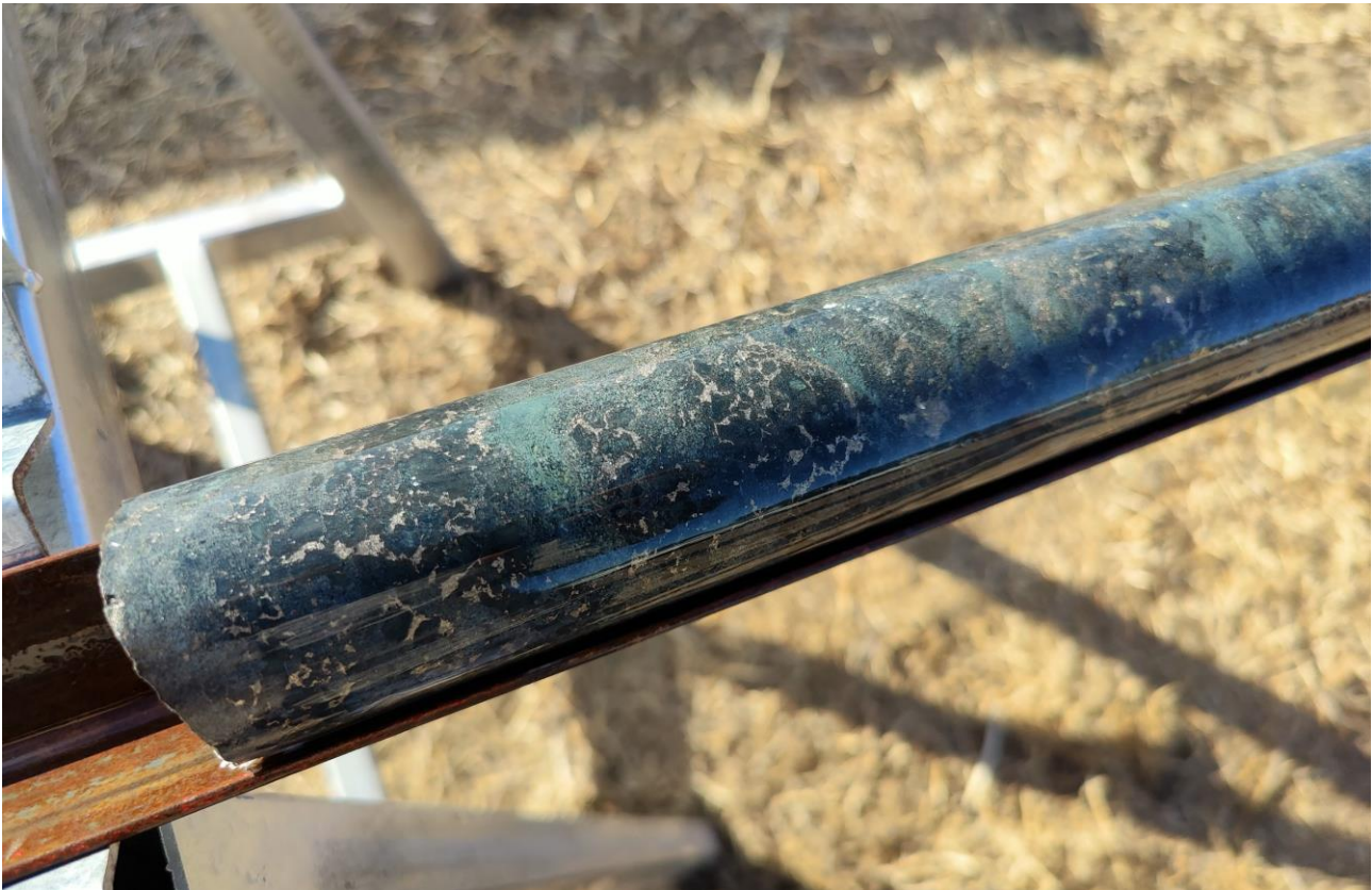
Figure 5. Interstitial sulphide mineralisation from the lower sulphide zone in YARCD0027 at approximately 253m.
