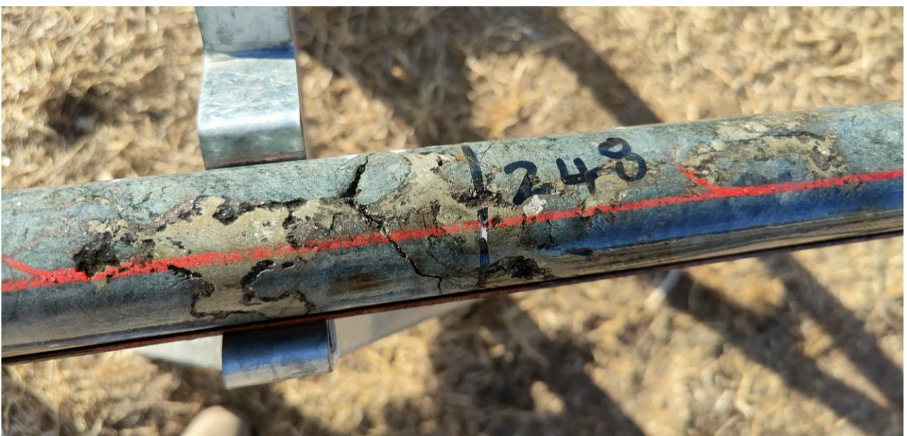
Figure 4. Coarse sulphide mineralisation (pentlandite-pyrrhotite +/- chalcopyrite), lower sulphide zone in YARCD0027 at approximately 248m.
