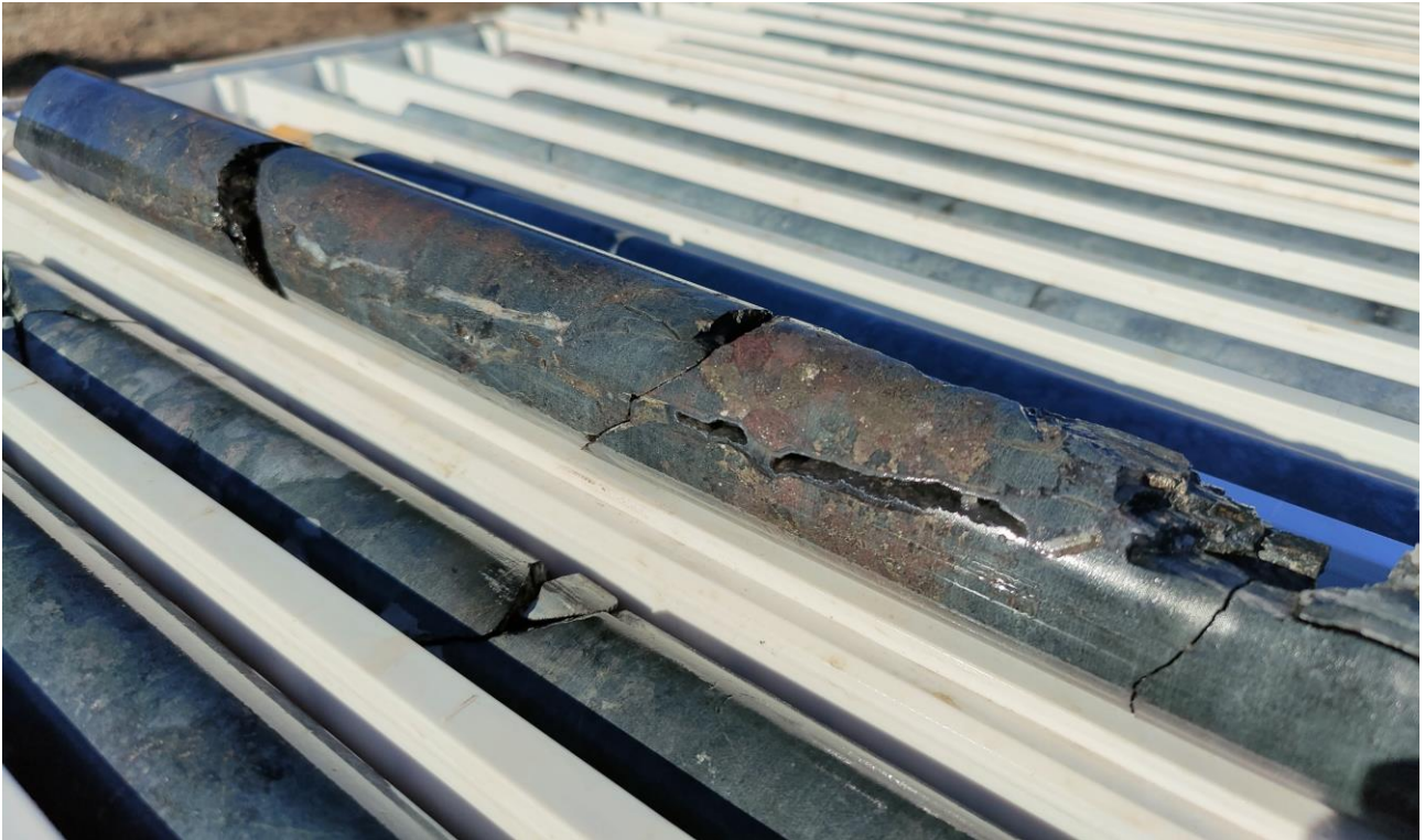
Figure 3. Sulphide mineralisation (pentlandite-pyrrhotite +/- chalcopyrite) and hematite alteration (red-brown mineral) in YARCD0025 from the upper sulphide zone at approximately 202m.
