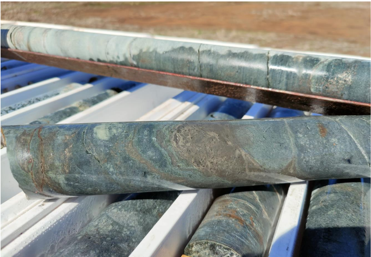
Figure 2. Shear and stringer sulphide mineralisation (pyrrhotite>pentlandite+/-chalcopyrite) within sheared and altered pyroxenite in YAD0024 at approximately 38m.
