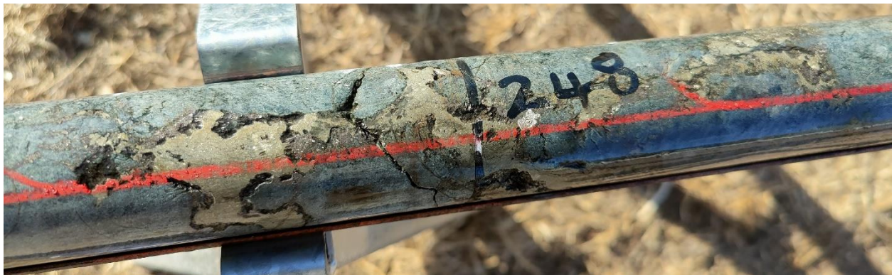
Figure 4. Coarse sulphide mineralisation (pentlandite-pyrrhotite +/- chalcopyrite), lower sulphide zone in YARCD0027 at approximately 248m.
