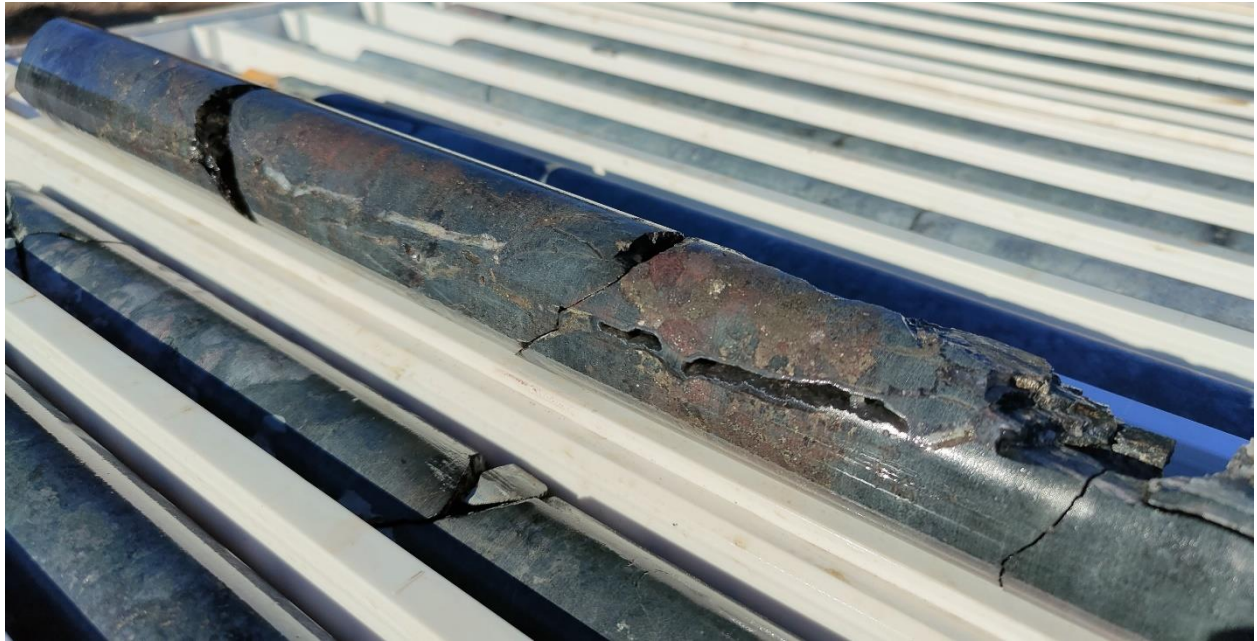
Figure 3. Sulphide mineralisation (pentlandite-pyrrhotite +/- chalcopyrite) and hematite alteration (red-brown mineral) in YARCD0025 from the upper sulphide zone at approximately 202m.
