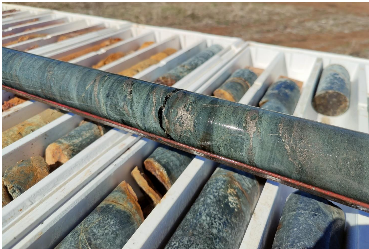
Figure 8. Shear and stringer sulphide mineralisation (pyrrhotite>pentlandite+/-chalcopyrite) within altered pyroxenite in YAD0024 at approximately 60m.
