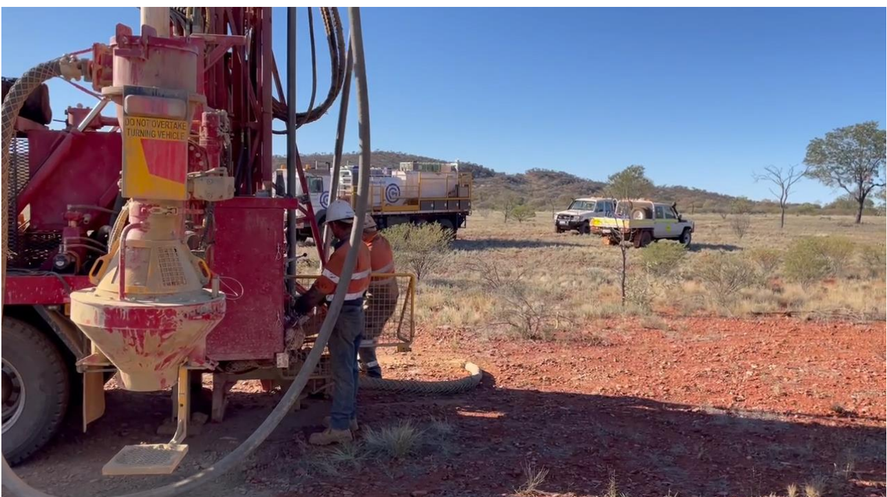
Figure 4. Aircore drilling at the Duchess Prospect, July 2022
