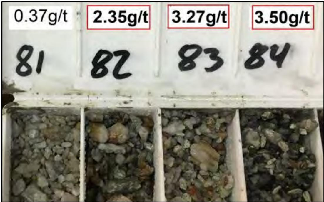
Figure 4: Hole KWGLRC02 81-84m rock chips (3m @ 3.04g/t Au)
