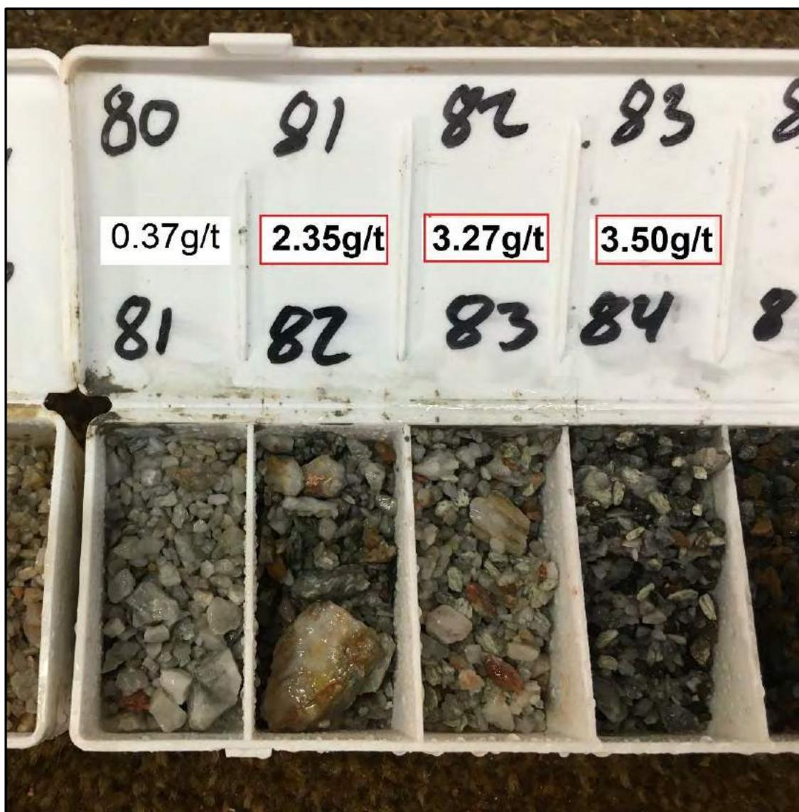
Figure 16: Hole KWGLRC02 81-84m (3m @ 3.04g/t Au)
