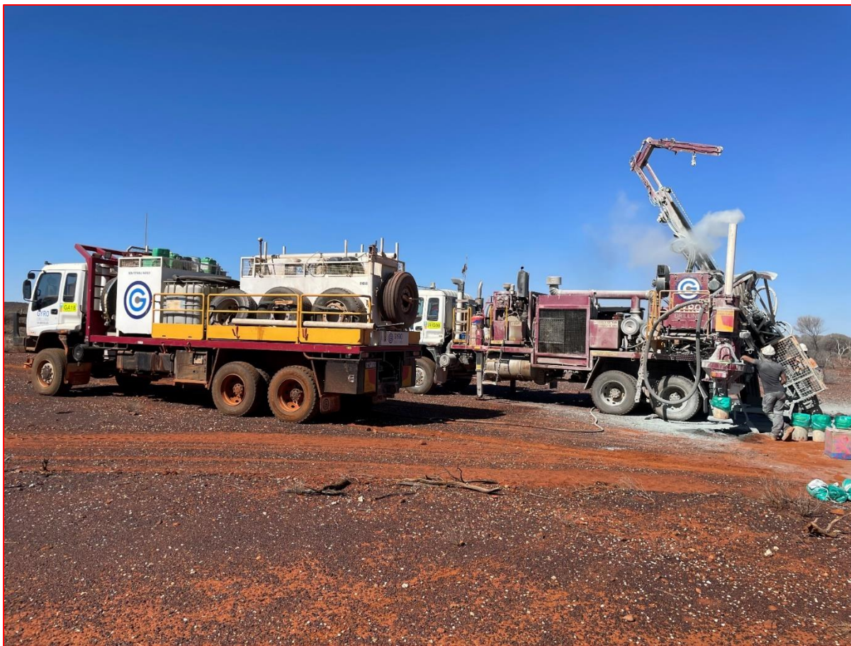
Figure 1: Reverse Circulation Rig Testing New Targets on the North of the Crawford Lease
