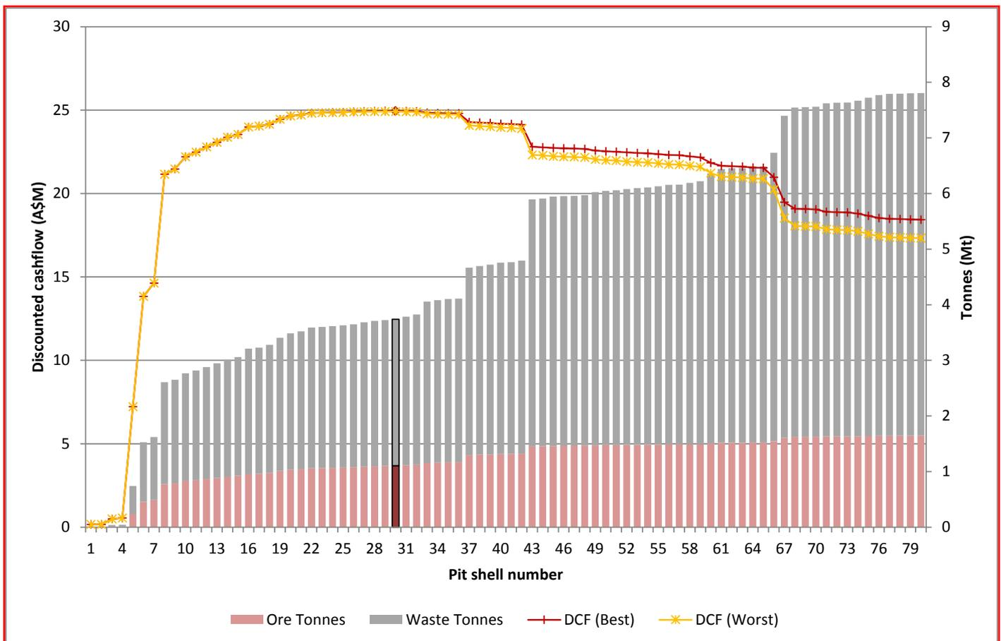
Figure 3: Crawford Oxidised Material Base Case Pit by Pit Graph
