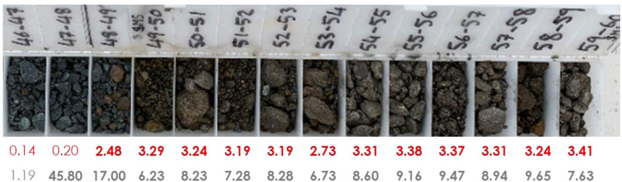
**Figure 3.** JRC001 drill chips and Ni+Pd assays showing the start of the massive sulphide interval from 48m.
