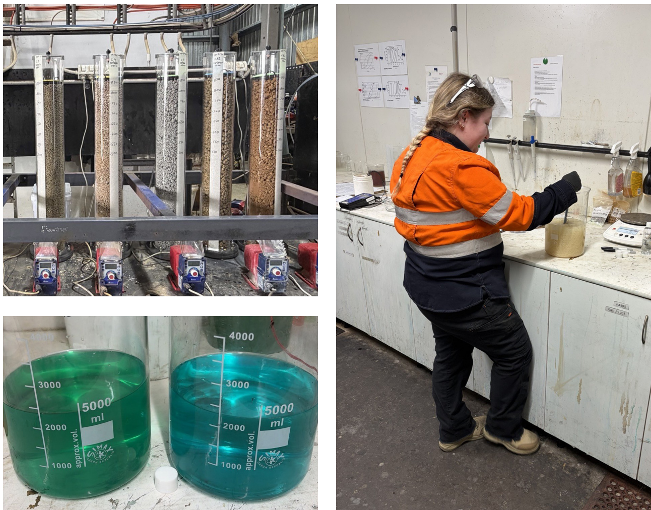
Figure 3 – Top left: Halls Creek leach columns at the Broken Hill Technology Centre. Bottom left: Leach liquor in contact with ion exchange resins. Right: Contacting leach liquor with ion exchange resin for silver recovery. Source: Cobalt Blue Holdings.
