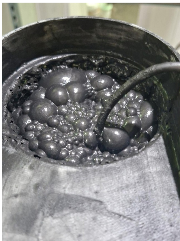
Figure 2 – Left: Column showing graphite (dark layer) selectively rising to the top during flotation, leaving behind gypsum (light grey layer) at the bottom – Right: Large, stable froth containing graphite. Source: Cobalt Blue Holdings.
