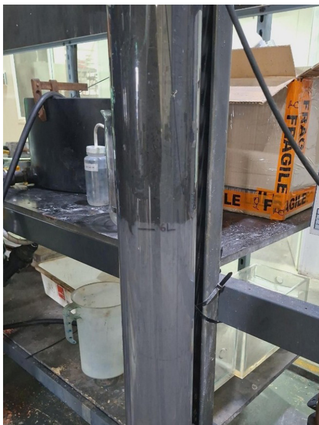
Figure 2 – Left: Column showing graphite (dark layer) selectively rising to the top during flotation, leaving behind gypsum (light grey layer) at the bottom – Right: Large, stable froth containing graphite. Source: Cobalt Blue Holdings.
