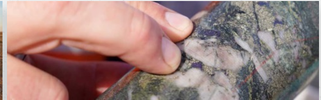
Quartz vein (15cm) with bornite (blue), pyrite and minor chalcopyrite at 221.2m
