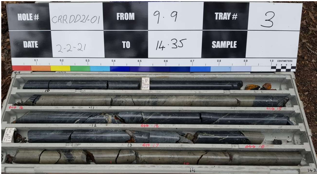
Figure 1. Core from 9.9m – 14.35m downhole, showing, in 2 nd row from top, a 0.85m massive sulphide interval (10.75m-11.60m with ~10% black carbonaceous shale) and, in the last row, the upper section of 3.8m massive sulphide interval (only ~ 14% black carbonaceous shales) that extends downhole from 13.3m-17.1m (Diamond drill hole CRRDD21_01, Scale: NQ core 50mm diameter variety)
