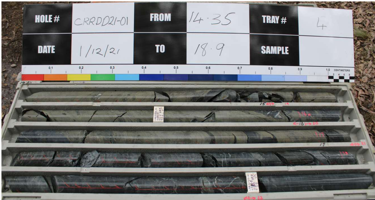
Figure 2. Core from 14.35m – 18.9m downhole, showing in the first three rows massive sulphide mineralisation that is part of a 3.8m interval (only ~ 14% black carbonaceous shales) extending from 13.3m-17.1m. (Diamond drill hole CRRDD21_01, Scale: NQ core 50mm diameter variety)
