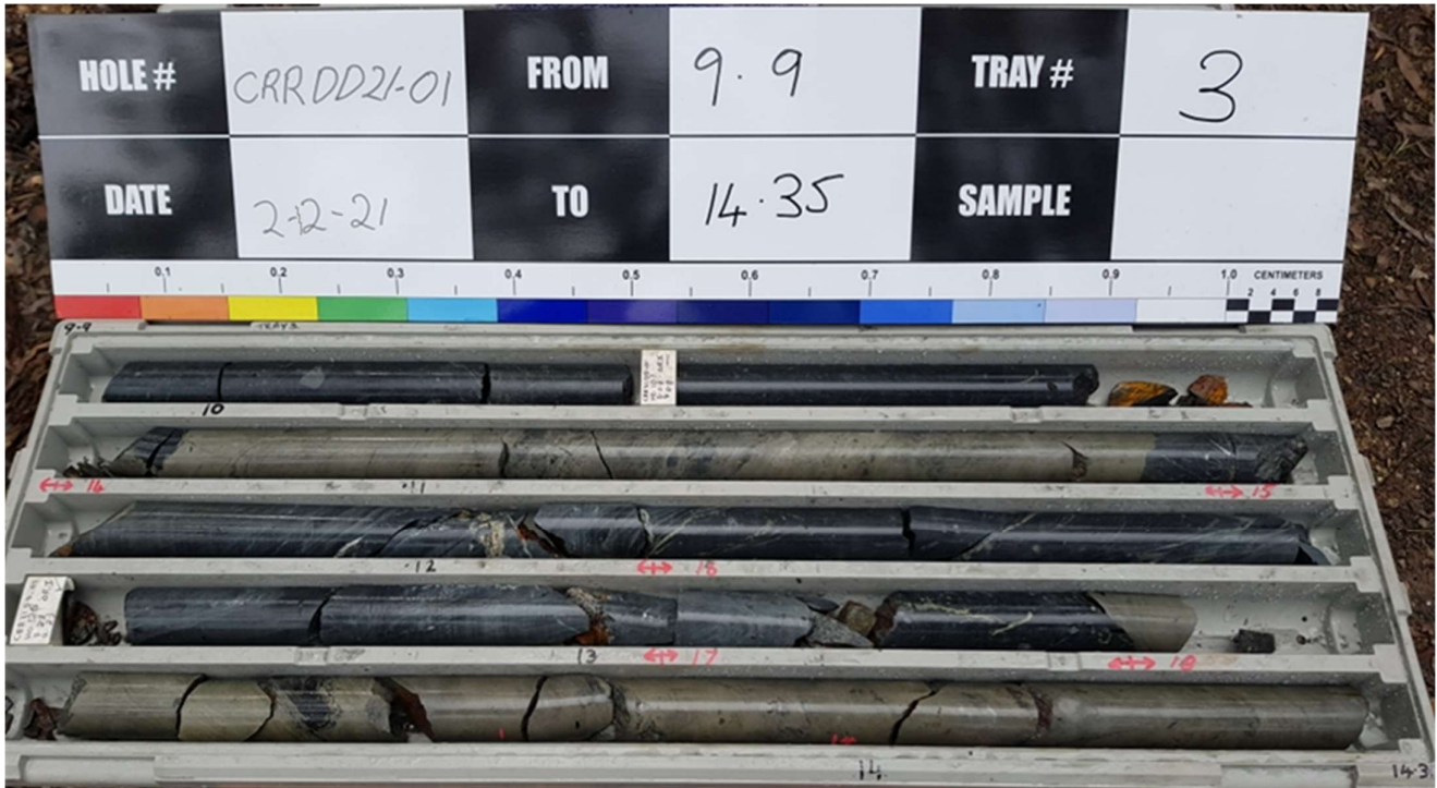
Figure 4. Core from 9.9m – 14.35m downhole, showing, in 2 nd row from top, a 0.85m massive sulphide interval (10.75m-11.60m with ~10% black carbonaceous shale) and, in the last row, the upper section of 3.8m massive sulphide interval (only ~ 14% black carbonaceous shales) that extends downhole from 13.3m-17.1m (Diamond drill hole CRRDD21_01, Scale: NQ core 50mm diameter variety)
