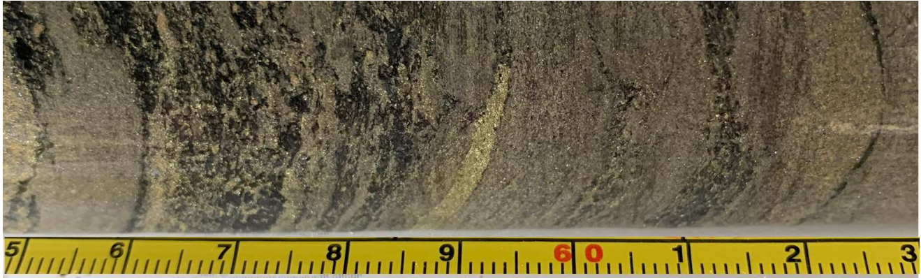
Figure 4. Core from 9.9m – 14.35m downhole, showing, in 2 nd row from top, a 0.85m massive sulphide interval (10.75m-11.60m with ~10% black carbonaceous shale) and, in the last row, the upper section of 3.8m massive sulphide interval (only ~ 14% black carbonaceous shales) that extends downhole from 13.3m-17.1m (Diamond drill hole CRRDD21_01, Scale: NQ core 50mm diameter variety)
