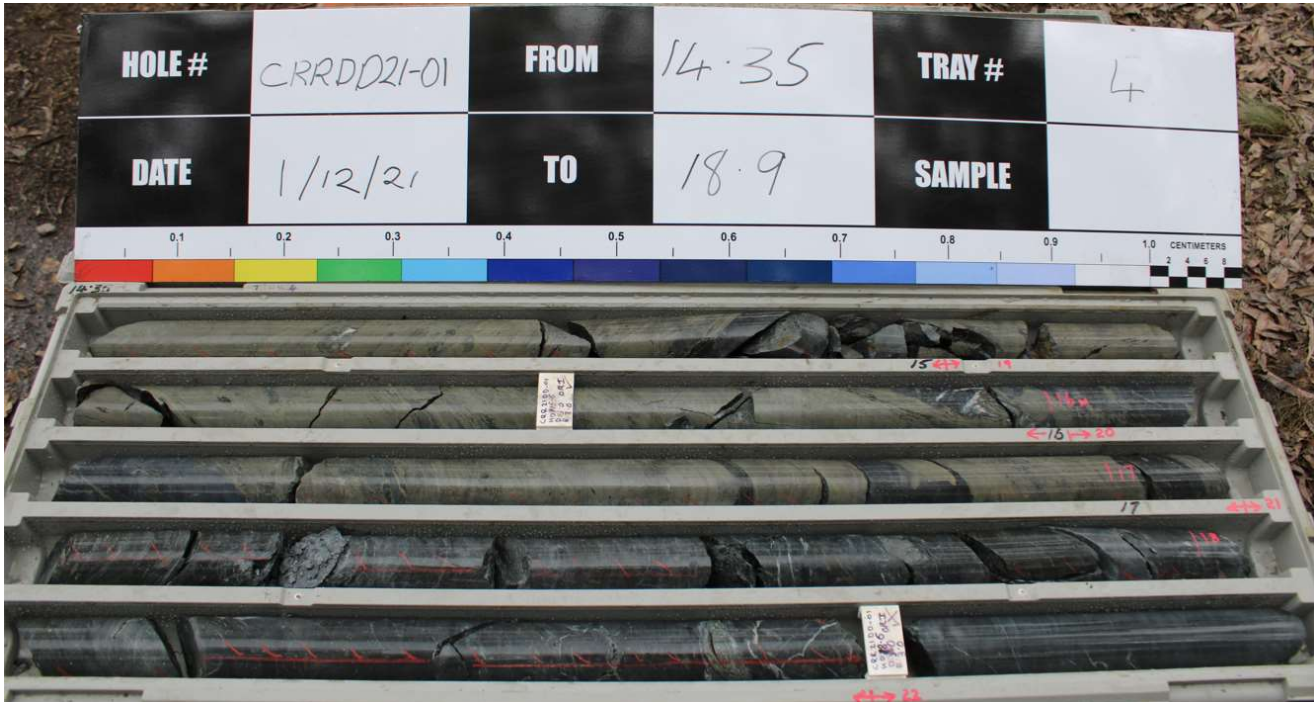
Figure 5. Core from 14.35m – 18.9m downhole, showing in the first three rows massive sulphide mineralisation that is part of a 3.8m interval (only ~ 14% black carbonaceous shales) extending from 13.3m-17.1m. (Diamond drill hole CRRDD21_01, Scale: NQ core 50mm diameter variety)
