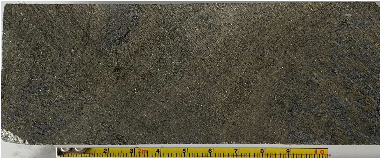
Figure 2: Detail of core from 102.8m-102.94m showing polymetallic mixed sulphides comprising sphalerite (Zinc), galena (Lead-Silver), chalcopyrites (Copper), (scale: centimetres)
