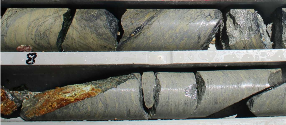
Figure 3: Detail of a shallow polymetallic massive sulphide interval that extends from 7.7m-9.6m downhole – Note yellow-brown low iron, high grade sphalerite (zinc sulphide) and silvery galena (lead sulphide) (Diamond drill hole CRR21DD_06, Scale: NQ core 50mm diameter variety)
