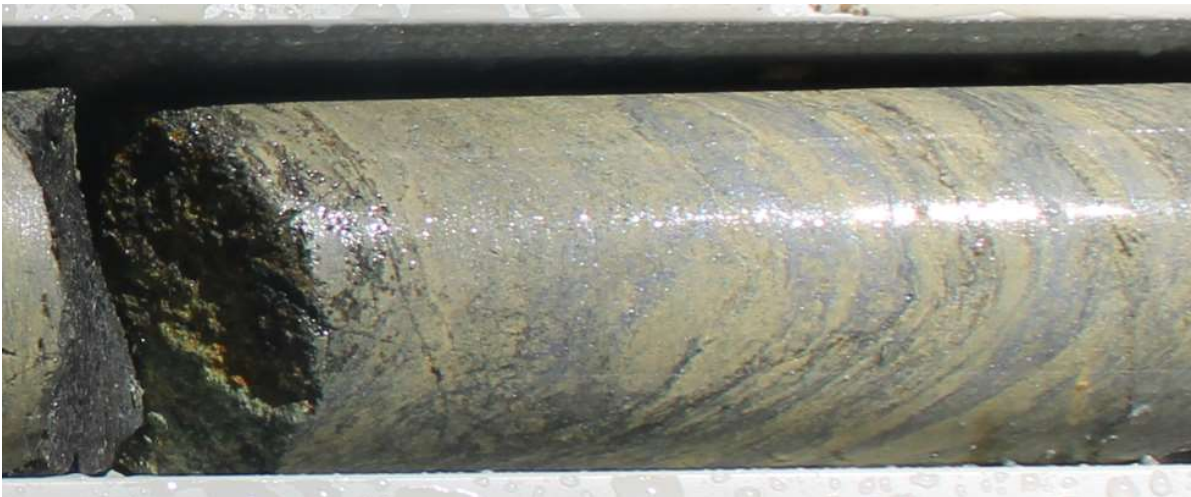
Figure 3: Detail of a shallow polymetallic massive sulphide interval that extends from 7.7m-9.6m downhole – Note yellow-brown low iron, high grade sphalerite (zinc sulphide) and silvery galena (lead sulphide) (Diamond drill hole CRR21DD_06, Scale: NQ core 50mm diameter variety)
