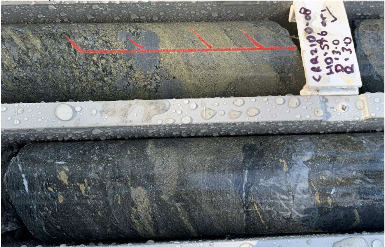
Figure 3: Disseminated sulphide mineralisation present as yellowy-brown discontinuous foliations and blebs black carbonaceous pelites (interval ~ 27.8m-30.6m downhole) (Diamond drill hole CRR21DD_08, Scale: NQ core 50mm diameter variety)
