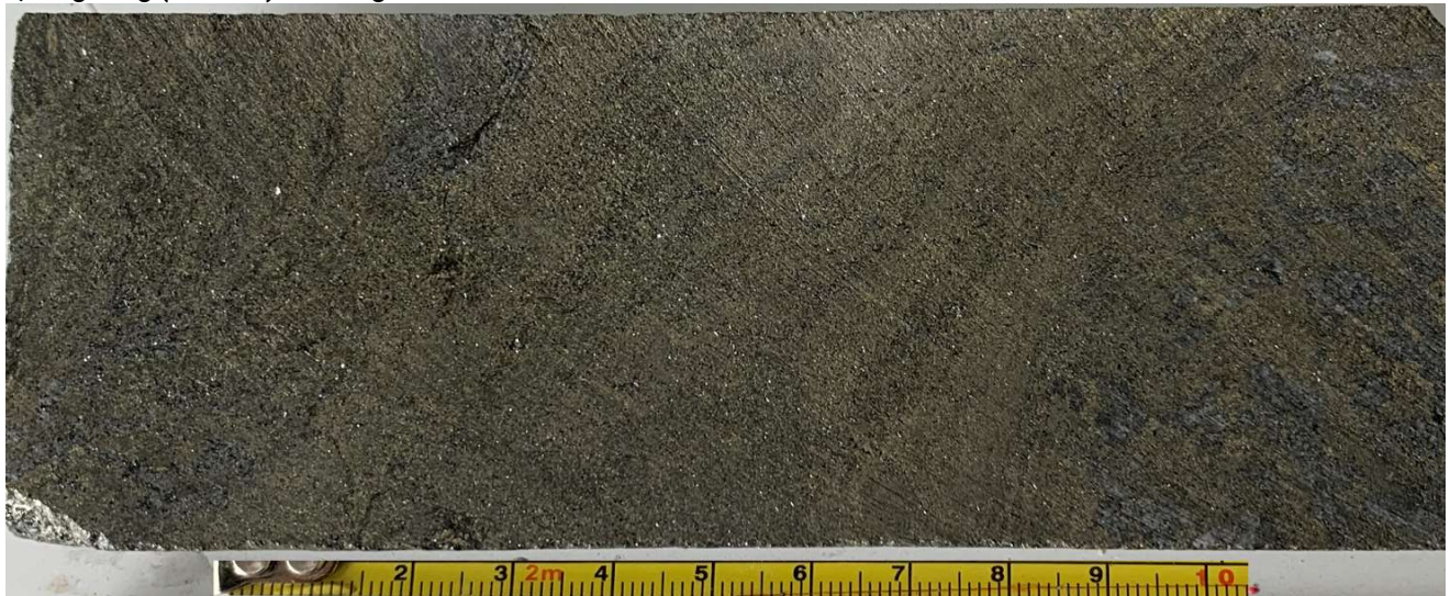
Figure 5: Detail of core from 102.8m-102.94m showing polymetallic mixed sulphides comprising sphalerite (Zinc), galena (Lead-Silver), chalcopyrites (Copper), (scale: centimetres). This interval assayed 22.00% Zn, 11.85% Pb, 3.84% Cu, 1,750g/t Ag (56.27oz) and 0.9g/t Au
