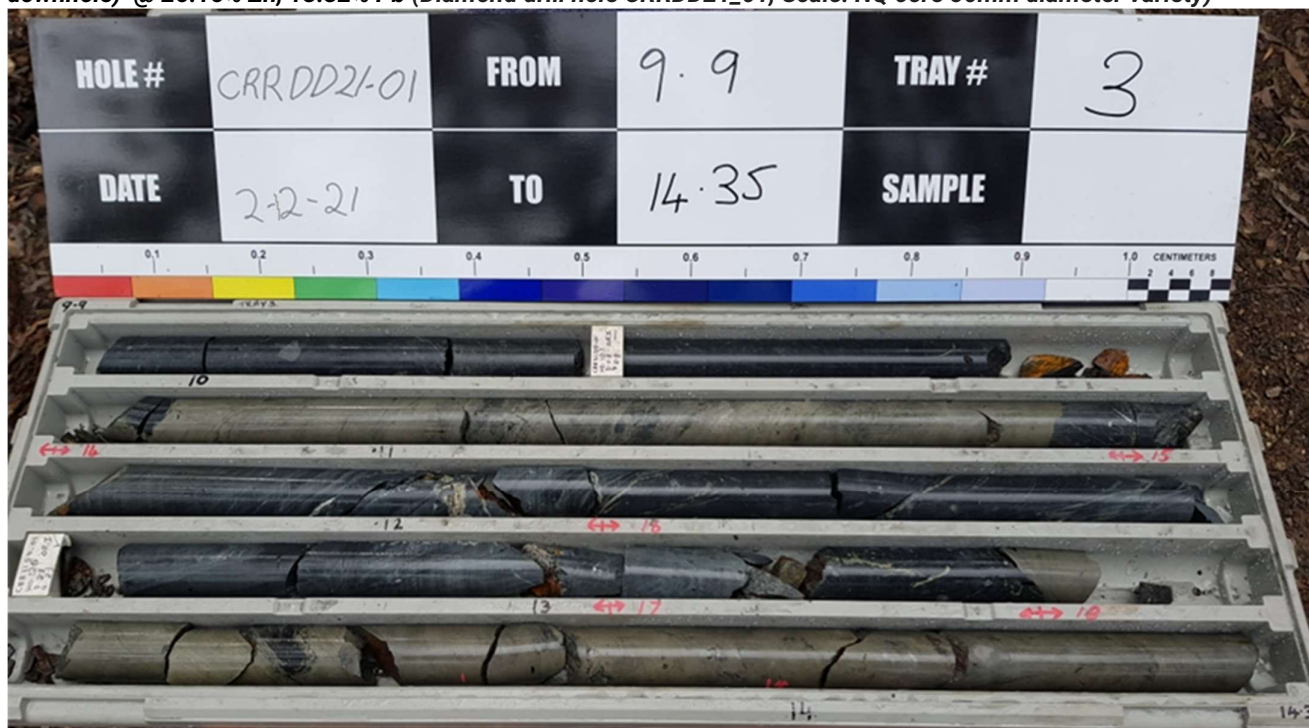
Figure 1: Core from 9.9m – 14.35m downhole showing in second and third rows 1.44m (from 10.75-12.19m downhole) @ 14.75% Zn, 7.93% Pb, 1.56% Cu, 571.95g/t Ag (18.39 oz) and 1.46g/t Au. Bottom row shows the upper (13.05m-14.35m downhole) portion of the high grade massive sulphide interval of 4.05m (from 13.05-17.10m downhole) @ 19.31% Zn, 10.23% Pb, 2.12% Cu 549.68g/t Ag (17.67 oz) and 1.89g/t Au – includes 2.1m (from 13.9-16.00m downhole) @ 25.15% Zn, 13.32% Pb (Diamond drill hole CRRDD21_01, Scale: NQ core 50mm diameter variety)
