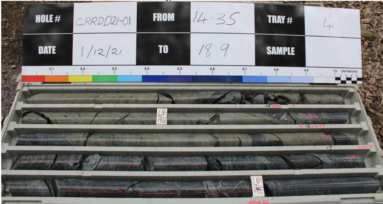
Figure 2: Core from 14.35m – 18.9m downhole, the upper three rows contain 2.75m of the 4.05m (from 13.05-17.10m downhole) of high grade massive sulphide interval that assayed @ 19.31% Zn, 10.23% Pb, 2.12% Cu, 549.68g/t Ag (17.67 oz) and 1.89g/t Au – includes 2.1m (from 13.9-16.00m downhole) @ 25.15% Zn, 13.32% Pb (Diamond drill hole CRRDD21_01, Scale: NQ core 50mm diameter variety)
