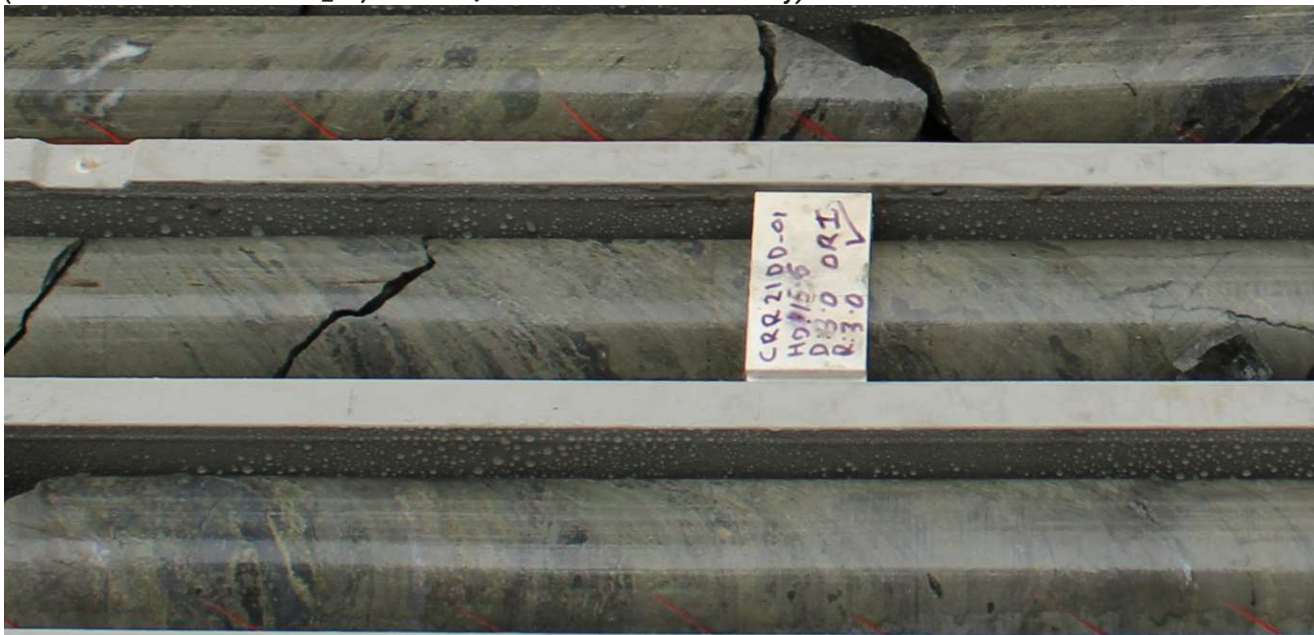
Figure 3: Detail of a section of the 4.05m high grade massive sulphide mineralisation shown in Figure 2 above (Diamond drill hole CRRDD21_01, Scale: NQ core 50mm diameter variety)
