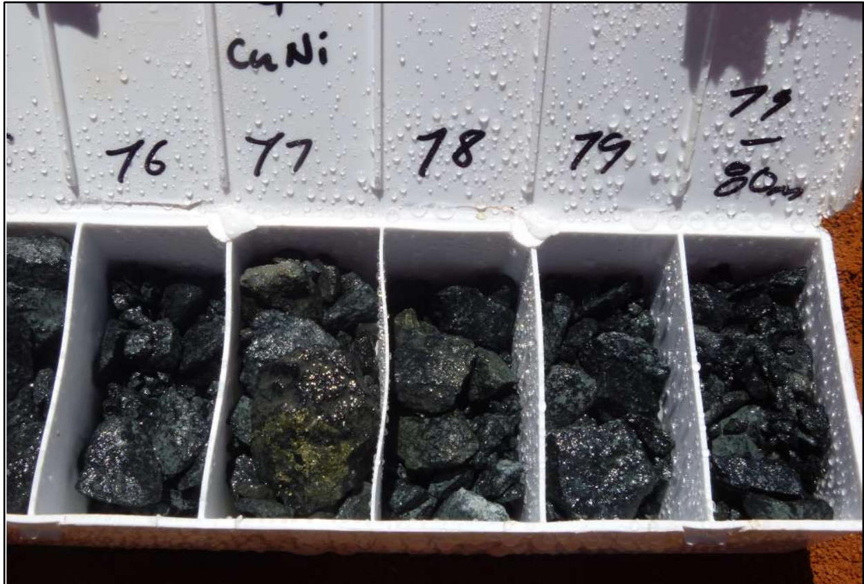
Image 2 / Stark chalcopyrite/pyrrhotite in RC chips, 76-80m NRC14007
