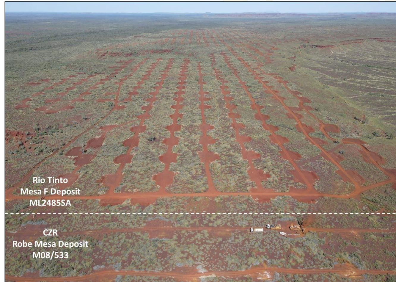
Boundary between CZR's Robe Mesa deposit and Rio Tinto's Mesa F deposit, showing recent drilling by Rio Tinto along the tenement boundary
