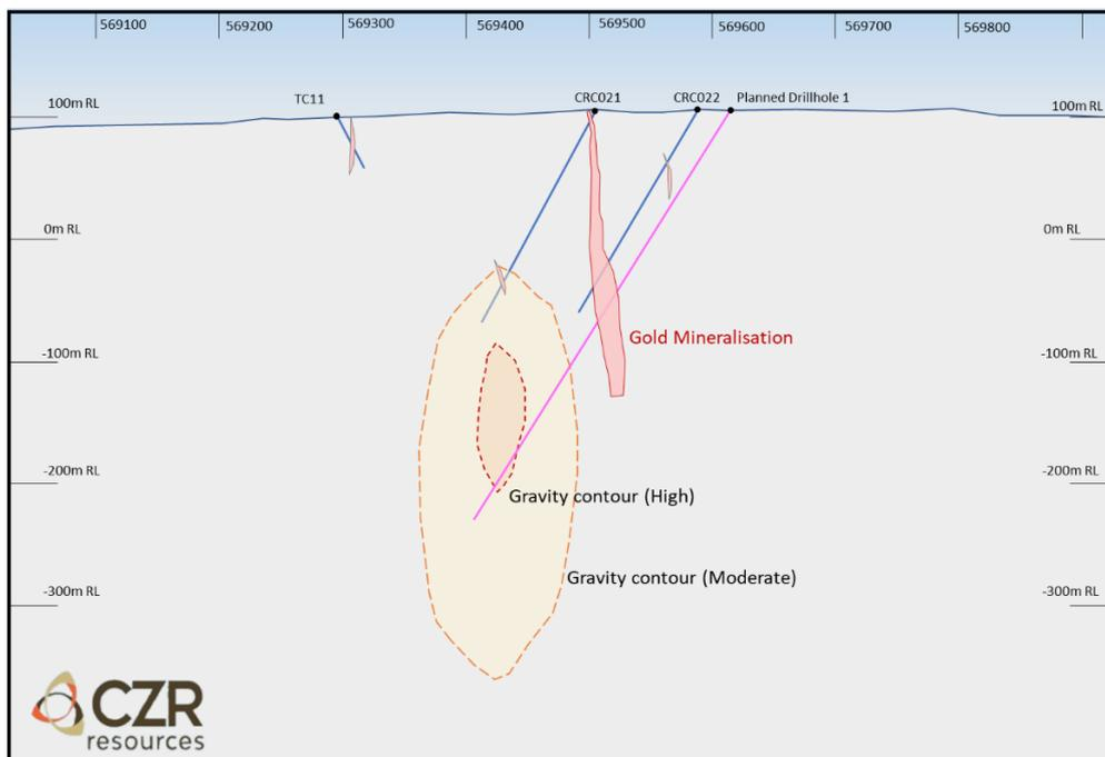
**Figure 14.** Top Camp Gravity inversion model – intrusion-related golds target (gravity high) with existing drill holes, primary gold mineralisation and planned drill hole
