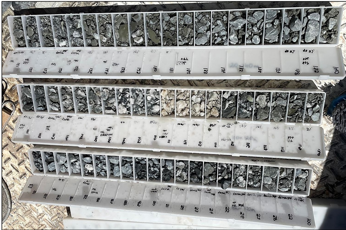
Figure 4. RC chip tray of hole CRC040 displaying wide zone of sericite-chlorite-pyrite alteration associated with quartz veining from 90-129m downhole, including a thick predominately quartz vein from 111-114m.
