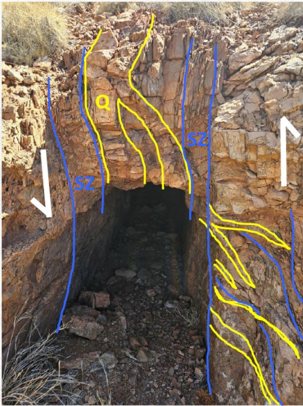
Figure 3. Adit portal at Top Camp exposing branching shear vein (looking southwest)
