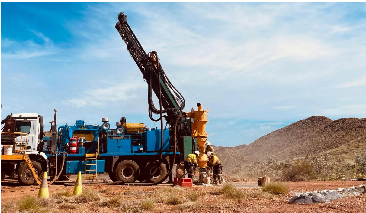
Figure 2. RC drilling underway at Top Camp – Croydon Gold Project
