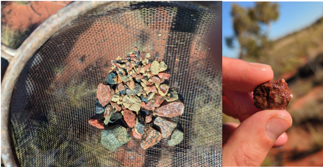
Figure 5. Gabbro and hematite altered quartz-feldspar intrusions from 26YRAC012.
