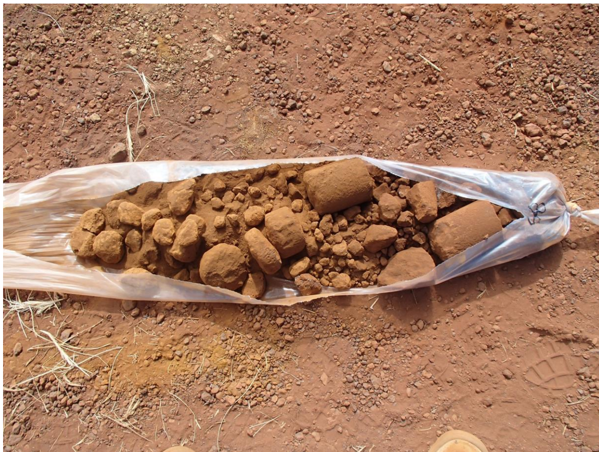
Fig 2. Samples of pisolitic iron-stone recovered by the sonic-rig from the Robe Mesa Deposit for the metallurgical test-work programme.
