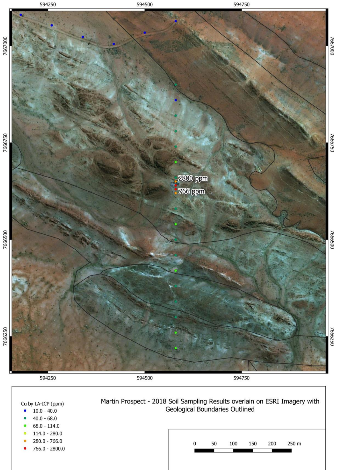
Fig 5. Distribution of copper (Cu) in soil from the first-pass orientation sampling over the mafic rocks hosting the Martin copper-zinc gossan overlain on the ESRI satellite imagery.
