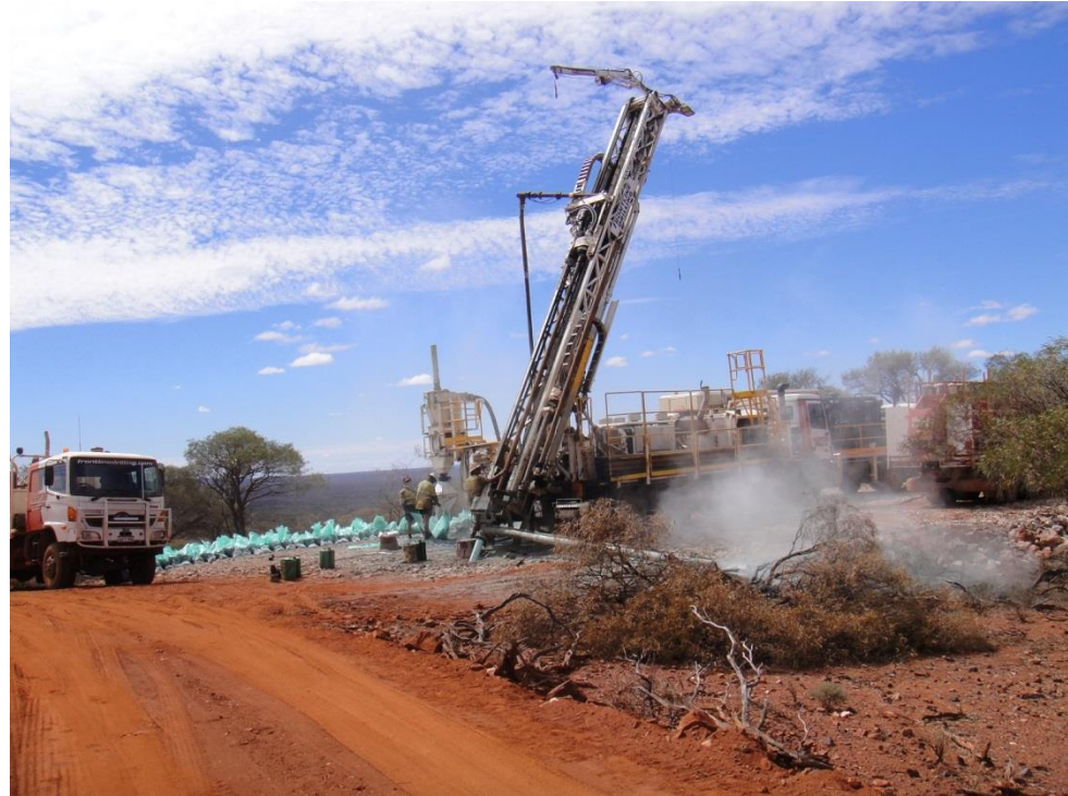
2018 RC drilling at the Buddadoo vanadium project
