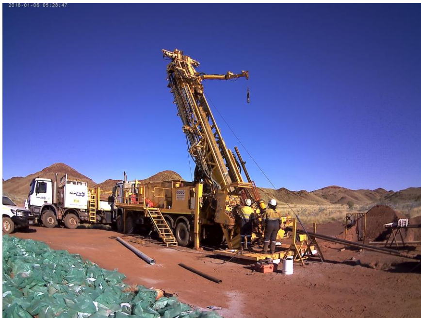
Fig 1 Topdrill diamond drill rig set-up near reverse circulation hole CRC007 at Top Camp.
