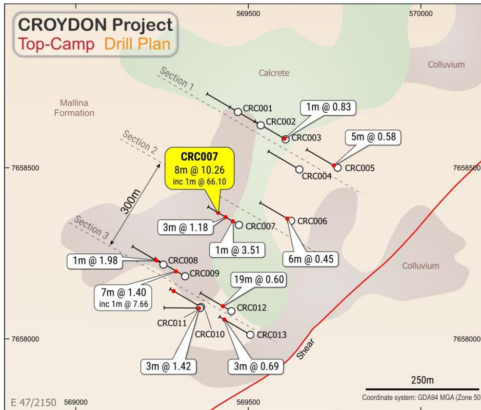
Fig 3 Location and down-hole traces of RC drill-holes CRC001 to CRC013 with significant intercepts in each drill-hole reported as metres at grams/tonne overlain on the Mt Wohler 1:100,000 geology.
