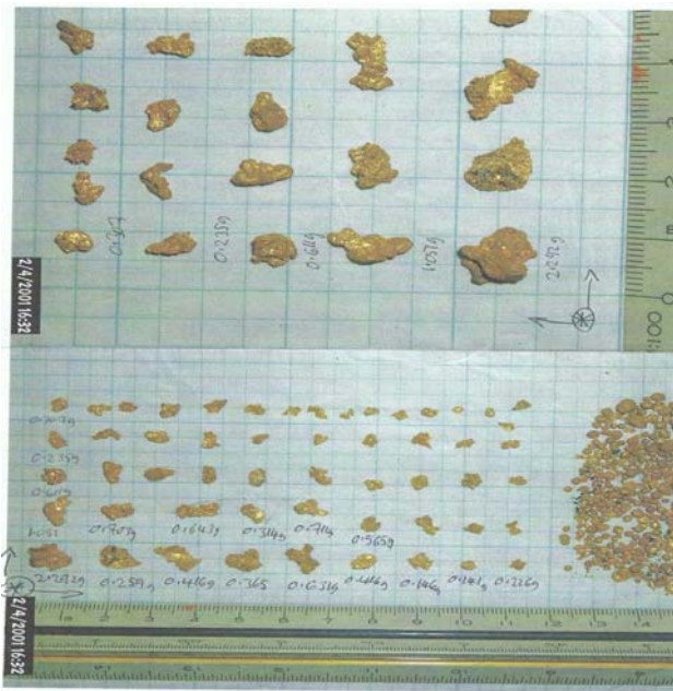
Photograph 3. 10kg Drill Sample - gravity recovered gold particles up to 2.29g in weight. Top image enlarged lower left area in bottom image.
