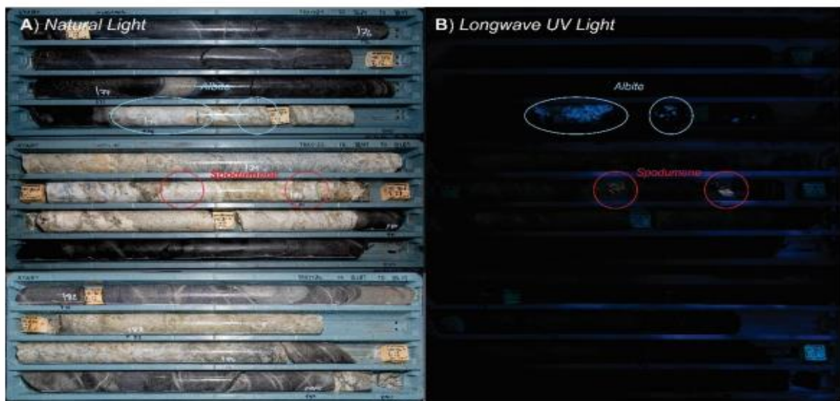
Figure 3 – Photographic compilation of the Fergusson pegmatite dyke in hole MIDDH005 under natural and longwave UV light, showing spodumene crystals in the core interval which assayed 0.62m at 1.63% Li 2 O. Also illustrated are large albite crystals, which demonstrates the megacrystic nature of some of these pegmatitic intervals.
