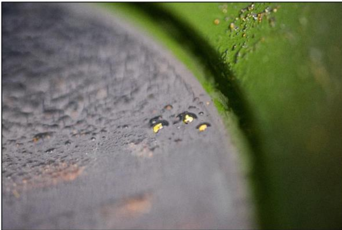
Figure 3 – Gold panned from a 0.4kg sub-sample collected from drilled interval 18 – 19m in RDRC03, which assayed at 7.0 g/t Au.
