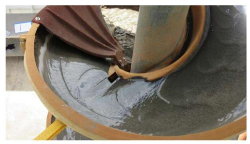
**Plate 2 –** Spiral separation of heavy minerals (dark grey colour toward centre) from lighter sand using a spiral bank
