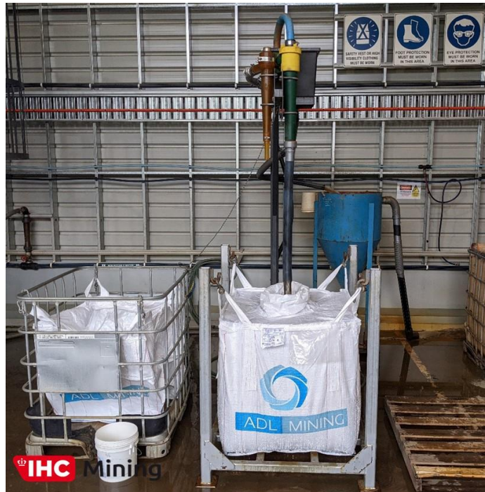
Plate 4 – Slimes removal (material <45µm)
