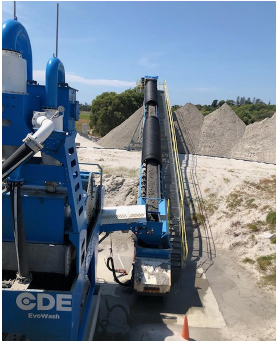
Plate 9 - Dewatered sand and movable stacker
