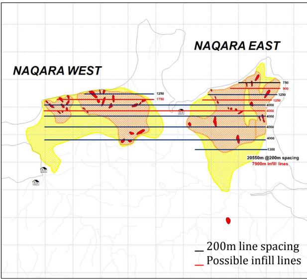
Figure 2 – Epithermal gold prospects (coloured areas) and proposed IP survey lines at Naqara, Ono Island, Fiji (grid lines are  $400 \times 400 \text{m}$ )
