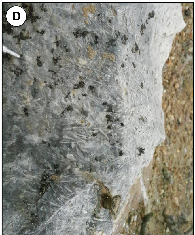
Figure 3: Photos from the Mia prospect showing typical (a) float trains of subcrop, including: (b) low temperature chalcidonic silica veins, and mineralised (c) banded and (d) bladed silica-sulphide veins.
