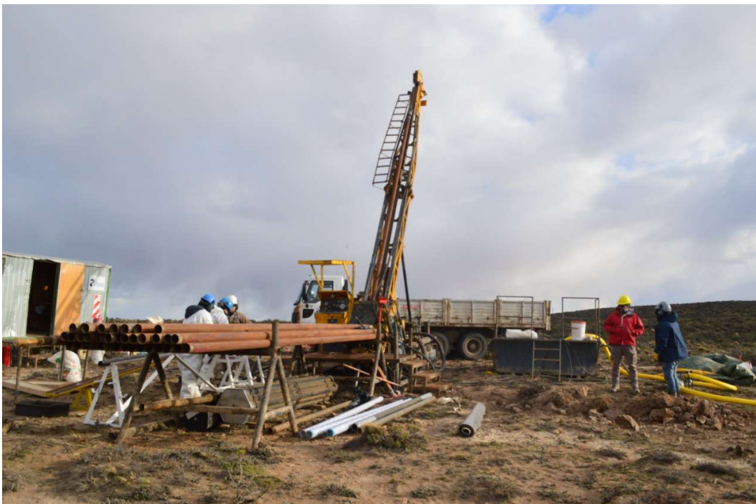
• Figure 2: Diamond drilling at the Mia Prospect
