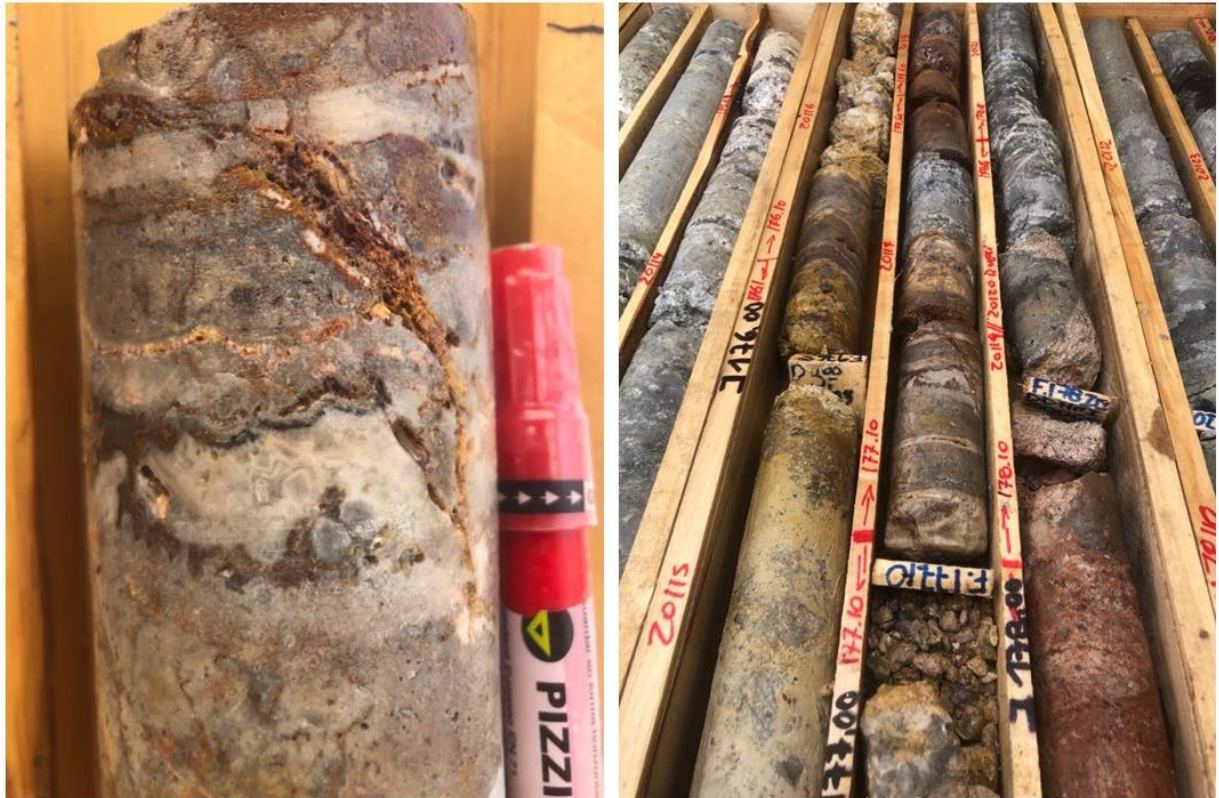
Figure 4: DDH-MI20-065, colloform crustiform epithermal vein from 175m
