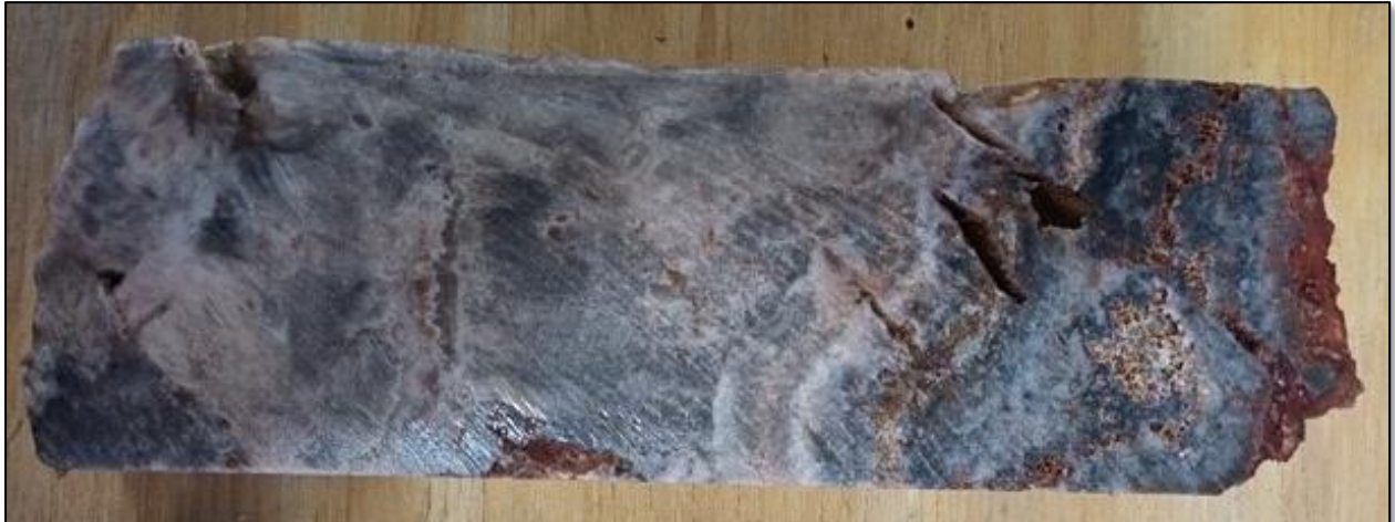
Figure 3: Hole CODD-114 epithermal vein from 71.4m with visible gold in vein selvages (shown below)
