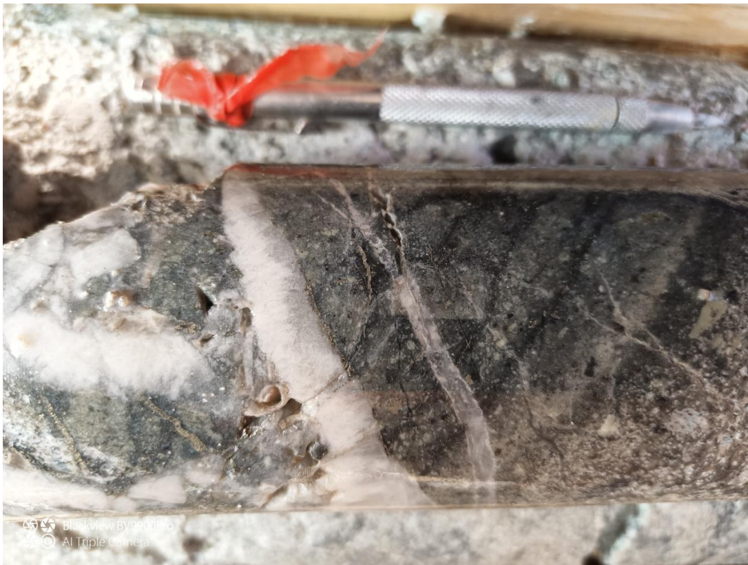
Figure 3: Hole CODD-125, close up of epithermal veins
