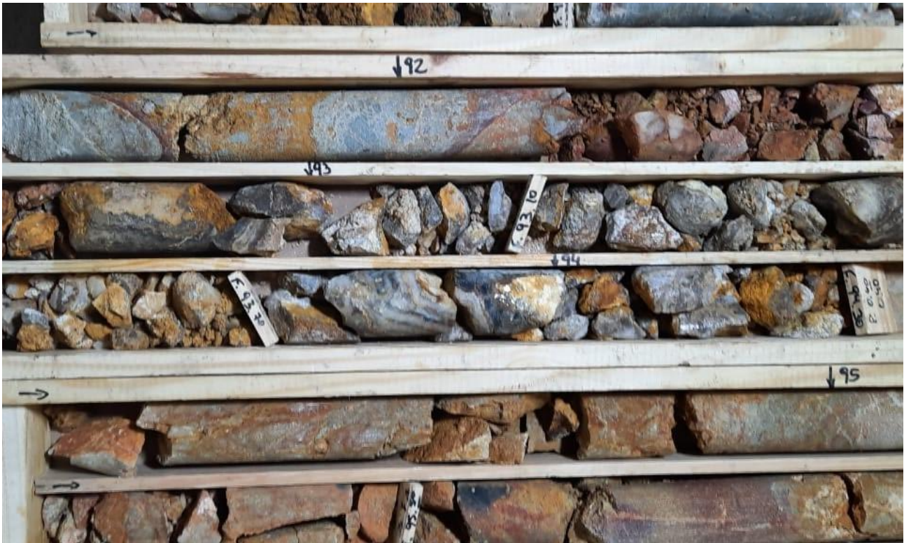
Figure 4: Banded epithermal veins – hole CODD-146 Malvina prospect
