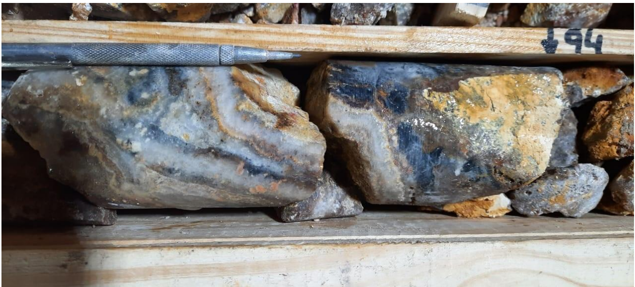
Figure 5: Banded epithermal veins – hole CODD-146 Malvina prospect
