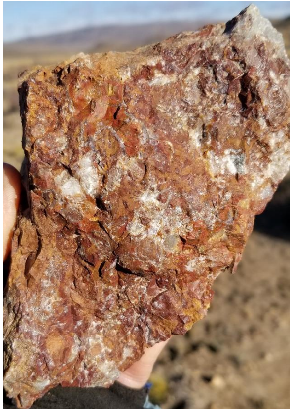
Figure 10: Jasperoidal silica breccia with thin crystalline quartz veins. 20gpt Au in rock samples
