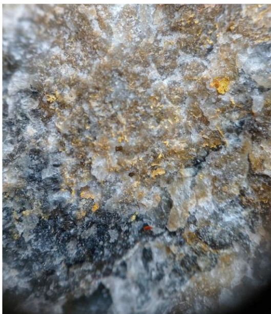
Figure 11: Visible gold (x10 magnification) in hand dug trench ROT-009 (1m at 279gpt Au, 116gp Ag)
