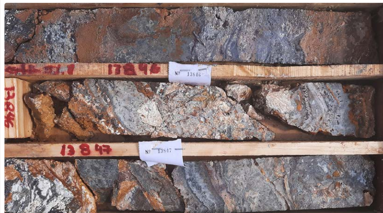
DDH-MI20-034: Colloform-crustiform vein
