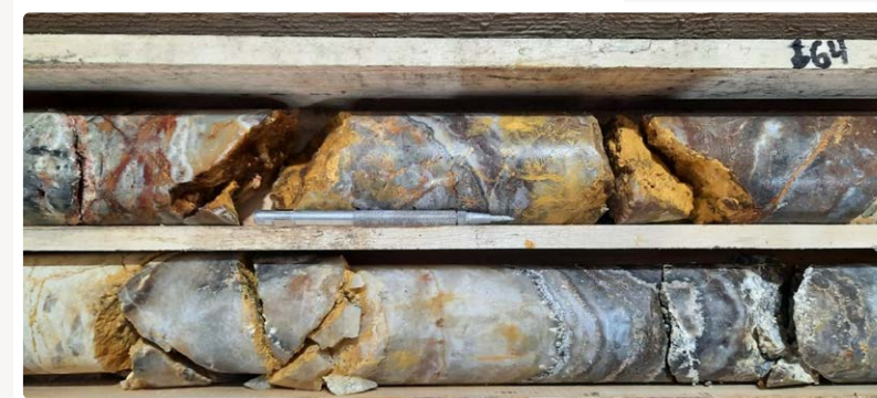
CODD-151: Colloform-crustiform vein
