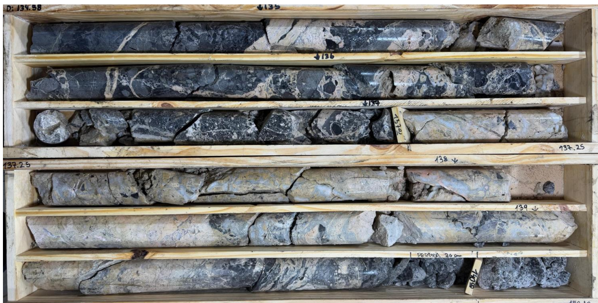
Figure 3: Hole P020-25 epithermal vein returning 4m at 2,400gpt AgEq (29gpt Au, 38gpt Ag)
